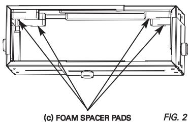
For large CPUs, attach foam spacer pads as shown in FIG. 1
